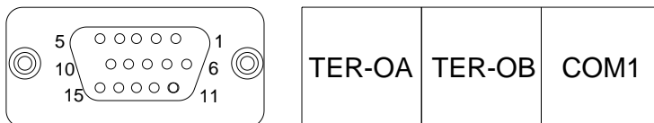
Figure A-12 PG card wire port and wire terminals
